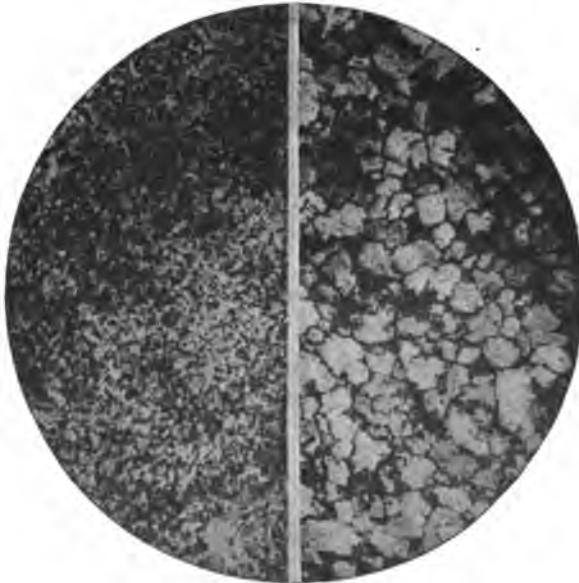
Fig. 6. Left: Casehardened Steel, Core, 0.03 Per Cent of Sulphur; Right: 0.06 Per Cent of Sulphur
